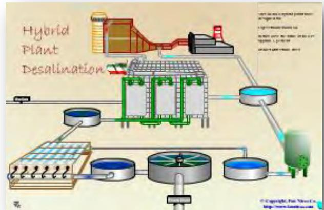
We have investigated an especial in which the brine discharge of BWRO units is recovered by a MED system. The hybrid elements are illustrated in the diagram above. This figure shows the main components and the connections between these elements.
